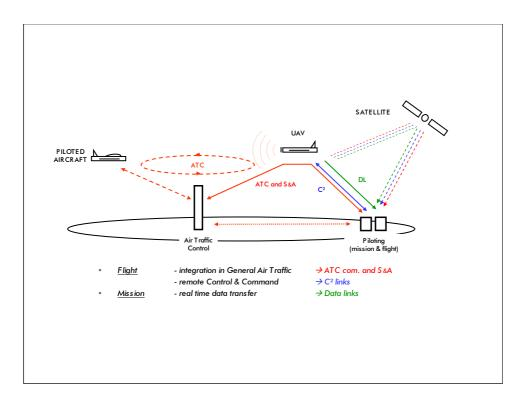
**Figure 1 : UAS communications and other functions**
