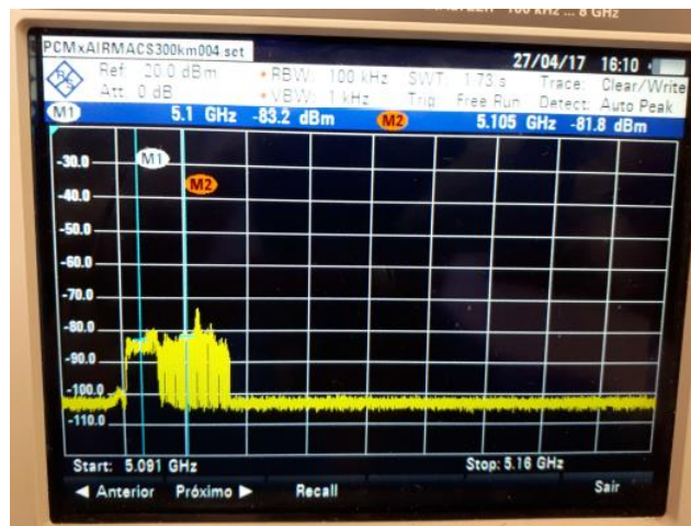
Figure 17: left side – AMT, right side – AeroMACS; Separation of 5MHz.
